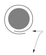
1/2 mil waxed Mylar around joiner rod, applied with vaseline
