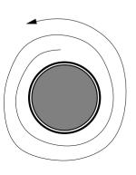
Spiral wrap with 1" wide 1 mil polyethylene strip (note direction)
